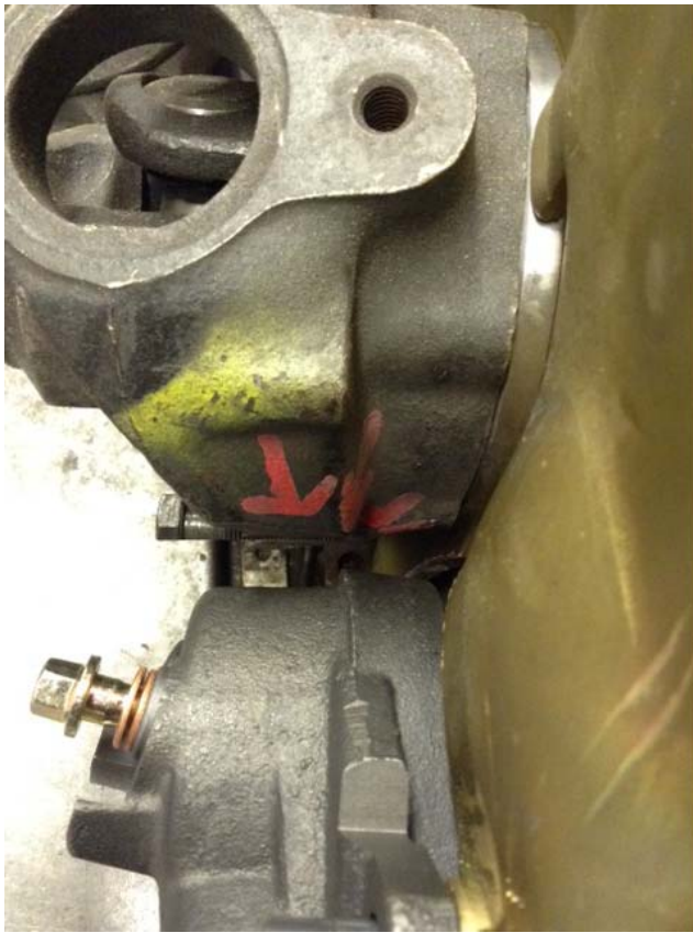
Figure 13: Caliper to Knuckle Clearance 1/8" Minimum Clearance
