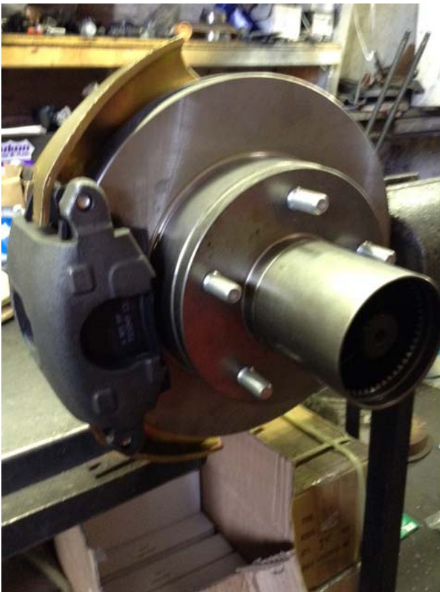
Figure 11: Installation of Disc Brake Caliper
