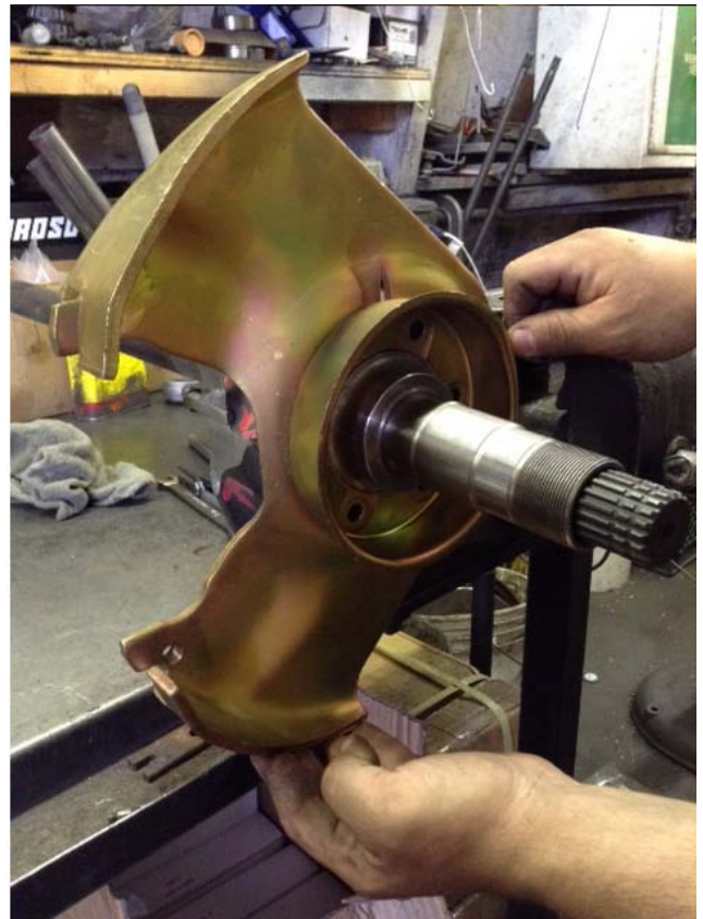
Figure 8: Installation of Backing Plate
