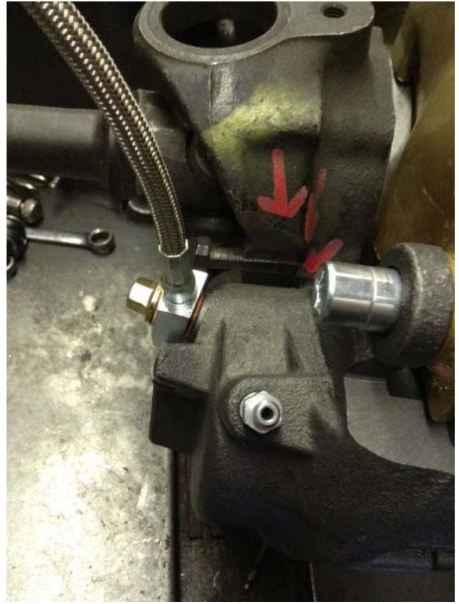
Figure 14: Brake Hose Installation – LINE UP
