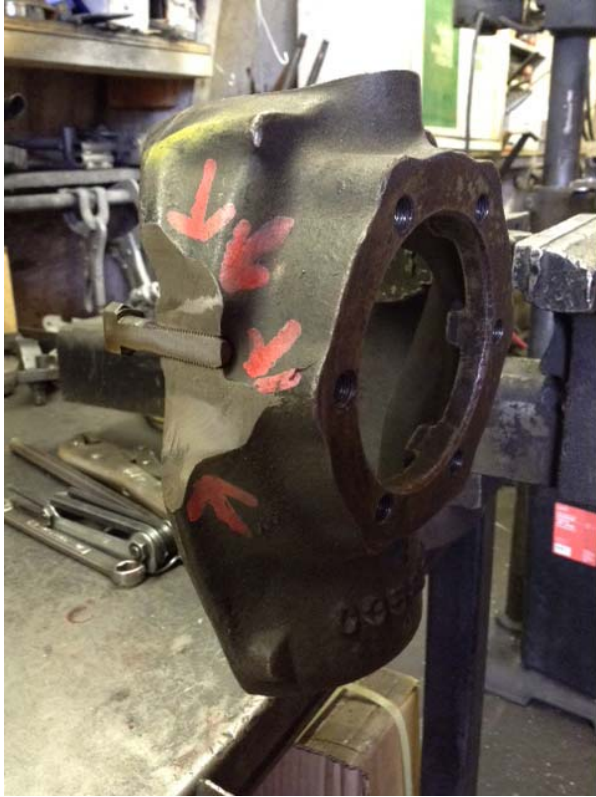
Figure 1: Grinding of Dana 44 Drum Brake Knuckle for Caliper Clearance
