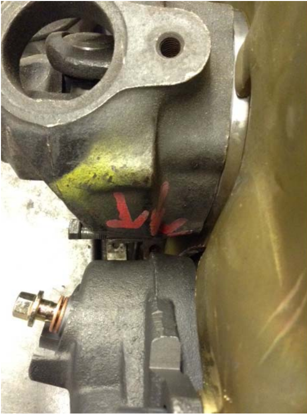
Figure 13: Caliper to Knuckle Clearance 1/8" Minimum Clearance
