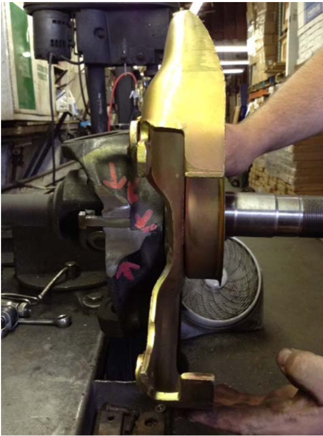
Figure 9: Installation of Backing Plate – Side View
