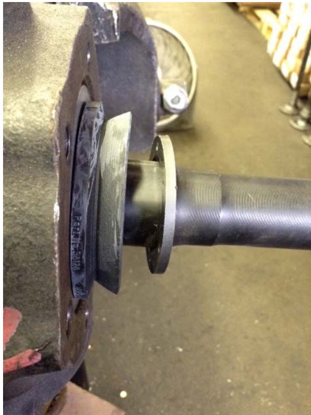
Figure 3: Installation of Thrust Washer (Inner Taper Facing Toward Knuckle)
