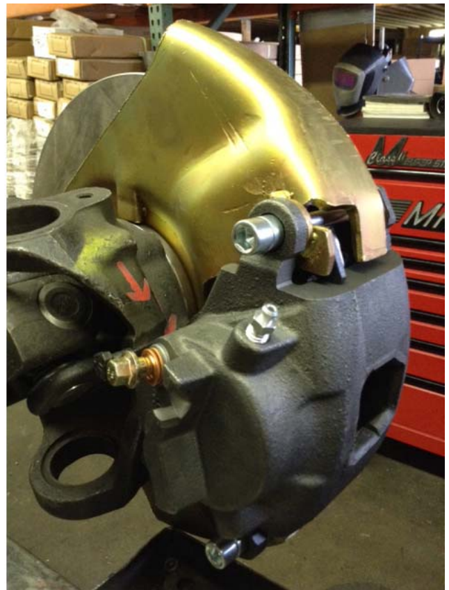
Figure 12: Installation of Caliper Bleeder Screw UP
