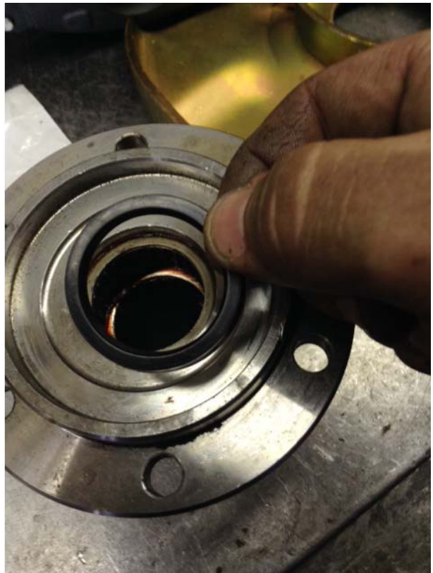
Figure 4: Installation of Spindle Bearing Cup Seal
