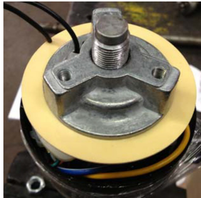
5. Install horn contact adapter plate.
