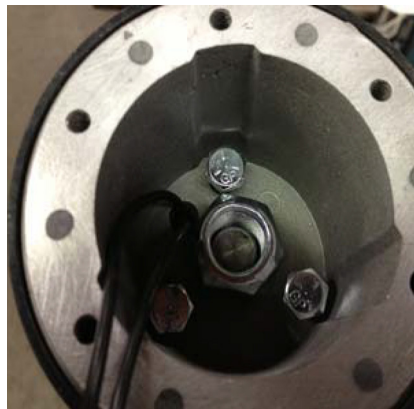
8. Install 3 shoulder bolts and column shaft nut.
