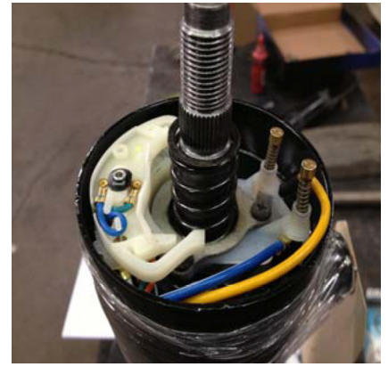
3. Install upper column shaft spring.
