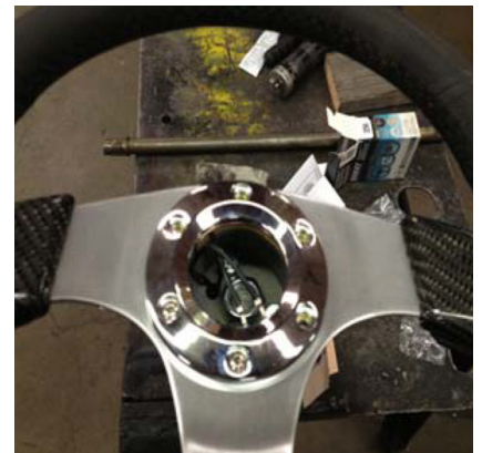
9. Align & install steering wheel to adapter.
