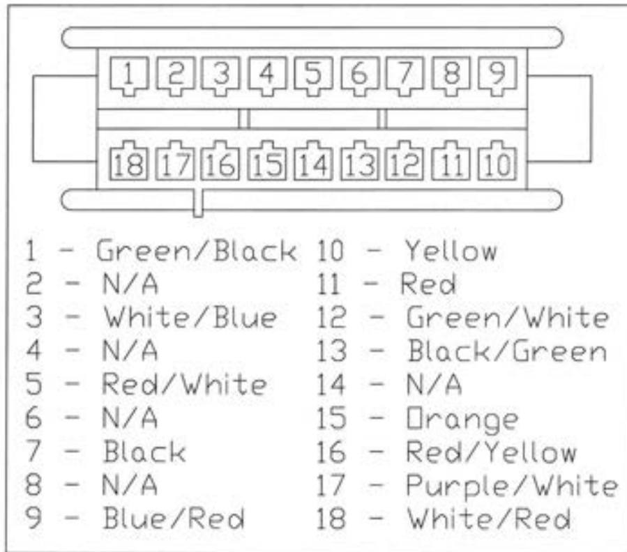
Figure 7-38 1973 - 1974 Cluster Pigtail Pinout
