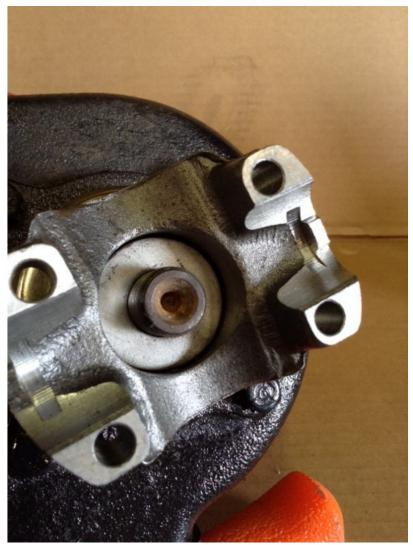
Install the Flat Washer (re-used from the old yoke).
