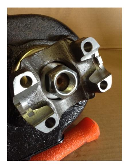
Install the nut and tighten down. The nut must be tight for proper preload of the bearings. Per the Ford Truck Shop Manual, this nut should be about 125-150 ft/lbs.
