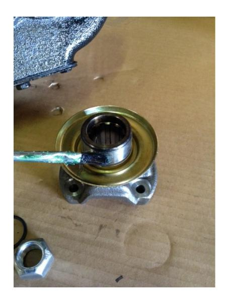
Apply a thin film of grease to the yoke where the seal will ride.
