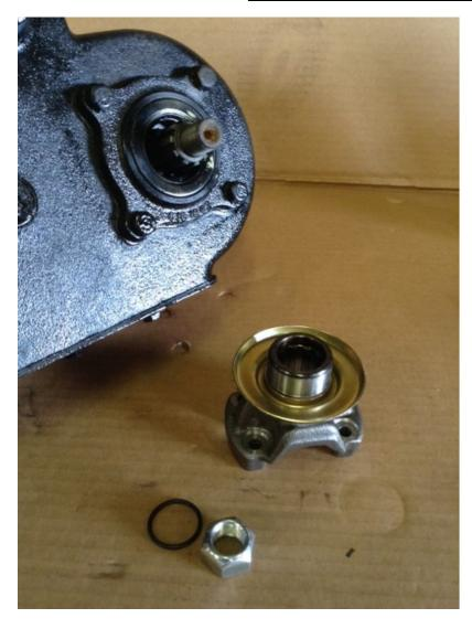
PARTS NEEDED: New Transfer Case Yoke, O-Ring, Top Lock Nut RE-USE: Yoke Flat Washer
